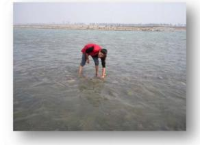
the flow of water. Samples were collected from about 30 cm depth after rinsing the sample containers with the river water. Field tests like colour, odour, temperature pH, ammonia, turbidity, conductivity DO, phosphate and colliform were performed at the site and sample containers were labeled properly for laboratory testing.
